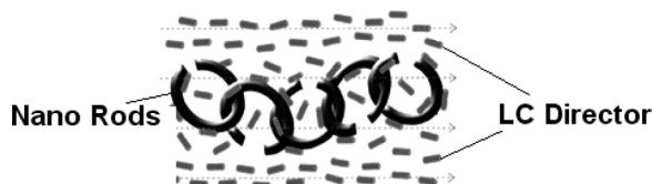
Figure 10. ZONPs (nanorods) in the nematic LC above the threshold field.
